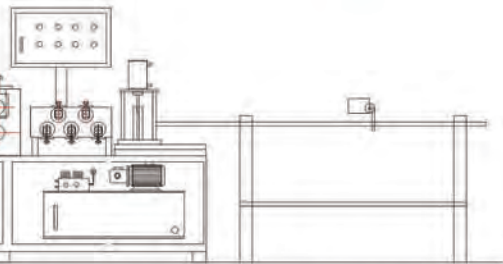
Straightening & Cut-off Run-out Table
